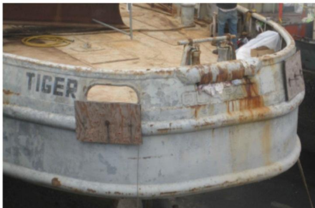
Rust and peeling paint
